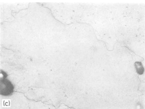
Figure 4 (a) Zn–Al alloy tested at 150° C (× 180), (b) Zn–Cu alloy tested at 150° C (× 180), (c) Zn–Cu alloy tested at 150° C (× 925).
